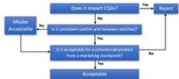
Figure 1: Decision tree used to accept or reject freeze-dried cake based on impact on CQAs (Patel et al., 2017).
