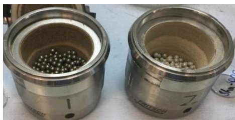
Figure 7: Sample vials after milling in the planetary ball mill for 30 mins at 400rpm, with 90 g of balls with 4 mm diameter. Left is with sodium hydroxide catalyst and right is sodium percarbonate catalyst.
