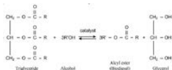
Figure 1. Transesterification of Triglycerides. Figure reproduced from Energy Procedia 32 (2013) pp 64-73
