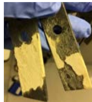
Figure 14: Rust-Oleum painted SS 304 (left) and SS 316L (right).
