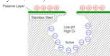
Figure 1: Pit formation. The positive symbols represent the cathodic region, whilst the negative symbols represent the anodic region under corrosive attack. (Misumi Technical Tutorial, 2010)
