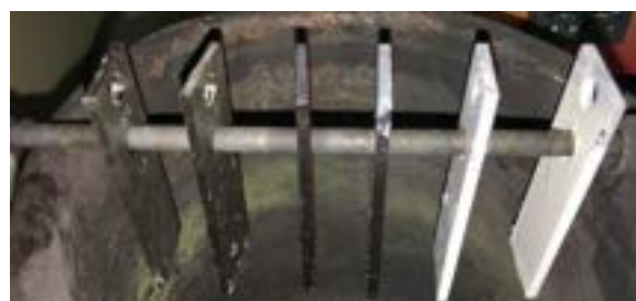
Figure 3: Coupon Set-up for the Furnace Experiments
