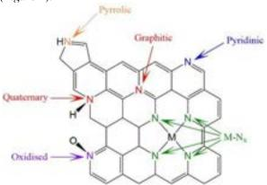
Figure 2: Different nitrogen moieties in N-doped graphene; the M- $N_x$  species are a result of further incorporating metal (M) atoms into the structure, adapted from Varela et al. <sup>10</sup>
