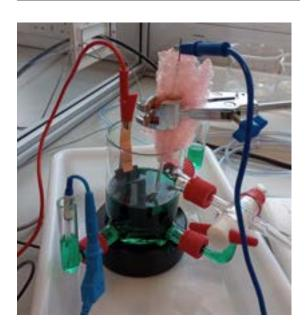
Figure 3: Electrodeposition setup involving an Ag/AgCl reference electrode (blue wire), FTO substrate as working electrode (red wire) and platinum counter electrode (black wire).
