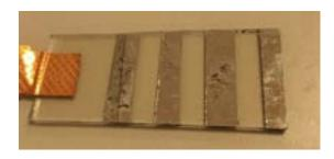
Figure 5: Nickel deposited on (2cmx4cm) FTO in grid structure as optimised by previous studies (Zhang, 2021).
