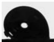
Figure 9. Photograph of a 10\mu\text{l} water droplet on a tablet surface tilted at 45^\circ
