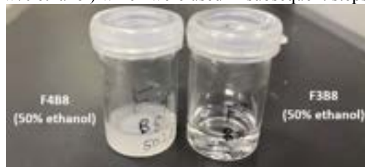
Figure 4.1. 3. 50 w/w% ethanol B8 added to F4 (left) and F3 (right). F4B8 turned cloudy whereas F3B8 remained colorless.
