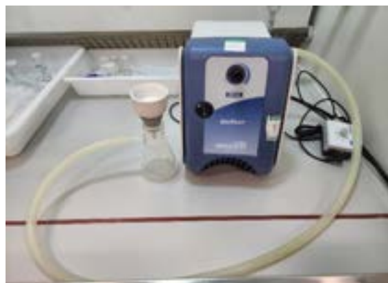
Figure 2. Filtration set-up depicting the Büchner funnel and flask (left), and the vacuum pump (right).
