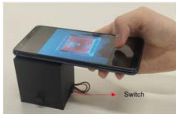
Figure 3: Operation of capturing images using the readout optical device. The magnified photographs on the top indicates the developed smartphone app for data collection and data analysis
