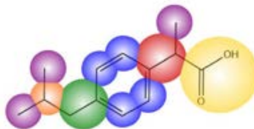
Figure 5. The molecular model used to model ibuprofen, image taken from (Wehbe, 2022). The molecular groups used to model ibuprofen were: 3 x CH_3 , 4 x aCH , 1 x aCCH , 1 x CCH_2 , 1 x CH , 1 x COOH . The ionised form of ibuprofen was modelled using the same groups as the molecular ibuprofen, the only difference is that the COOH group in molecular ibuprofen was replaced by the COO^- group in the ionised form.
