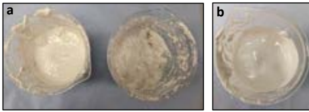
Figure 6a) Wet samples mixed with 3000 ppm FLOPAM FO 4650 VHM (left) and 2000 ppm FLOPAM FO 4650 VHM (right) b) Wet sample mixed with 7000 ppm FLOPAM FO 4650 VHM poorer consolidation of the \text{CaCO}_3 at high FLOPAM FO 4650 VHM doses. Qualitative observation reinforces this hypothesis, as samples with higher concentrations of secondary polymer were creamier and more homogeneous than those at lower dosages, indicating a breakdown of flocs during the high shear mixing process. A comparison of these samples before they were left to dry can be observed in Figure 6. The samples in Figure 6a have a lower amount of secondary cationic polymer (3000 and 2000 ppm from left to right) and are seen to still contain macroscopic flocs of aggregated \text{CaCO}_3 . The sample in Figure 6b contains 7000 ppm of secondary polymer, equal, which is well into the overdosing region of Figure 5 and its texture is much more uniform with no visible clumps of particles.
