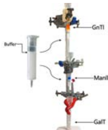
Figure 10. Establishment of Sequential Packed Bed Reactor with Immobilised Enzyme Cascade
