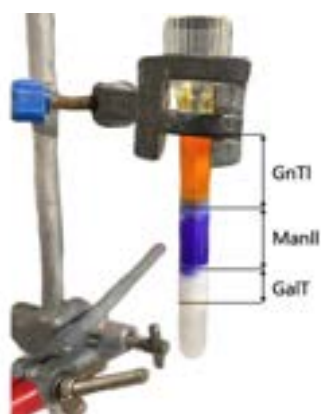
Figure 9. Establishment of Continuous Packed Bed Reactor with Immobilised Enzyme Cascade
