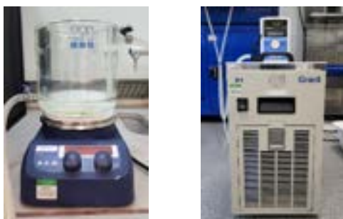
Figure 1. Experimental set-up depicting the glass vessel and magnetic stirrer (left), and the water bath (right).
