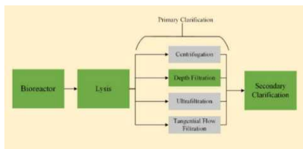
Figure 1: CFPS production process with primary clarification alternatives
