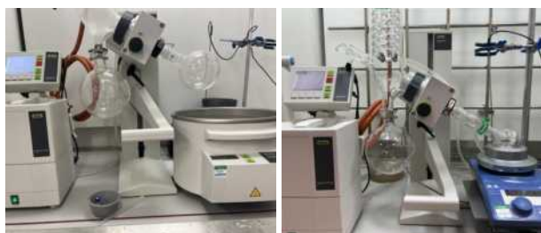
(a) Acetone Solvent System; operating conditions of 85°C and 50mbar, heated with a water bath (b) DMSO Solvent System; operating conditions of 220°C and 35 mbar, heated with a heating plate
