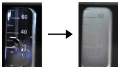
Figure 4. Camera Imaging of Vessel, with Solution Before and After the Occurrence of Nucleation
