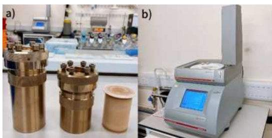
Figure 3: Equipment used for experiments. a) Two sizes of autoclaves and linear for synthesis. b) Microwave reactor
