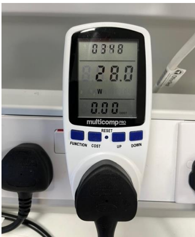
Figure 2: Single phase meter measuring power (W)
