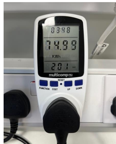
Figure 3: Single phase meter measuring energy (KWh)
