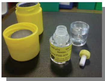
Packaging with a stopper (bottom right) designed to prevent contents from shifting during transit
