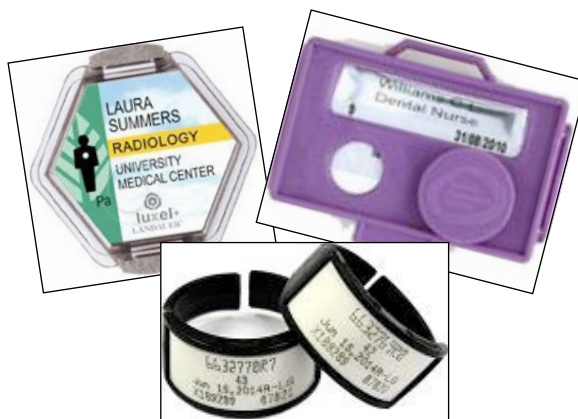
Examples of body and extremity (finger) dosimeters in use at Imperial College
