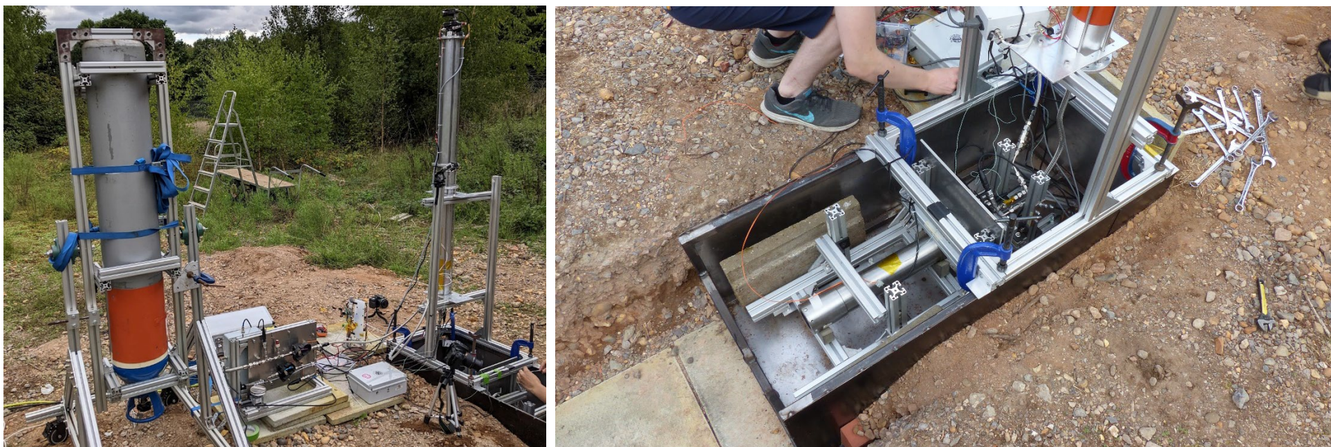
Figure 3: Images showing actual components to be used for hot fires. (left to right) The Tank Inverter with N 2 O cylinder, the Test Fire Box (with engine mounted) and the Run Tank. Not shown are the Nitrogen Cylinder (to be secured to a trolley) and the Methanol fuel tank stand (to be stood next to the test fire box).
