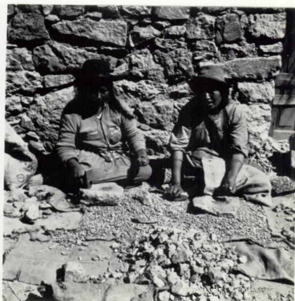
(20) Crushing - 20th Century style! Two Indian women crush bismuth ore at Belivar Bismuth mine, 25 miles from San Pablo.
