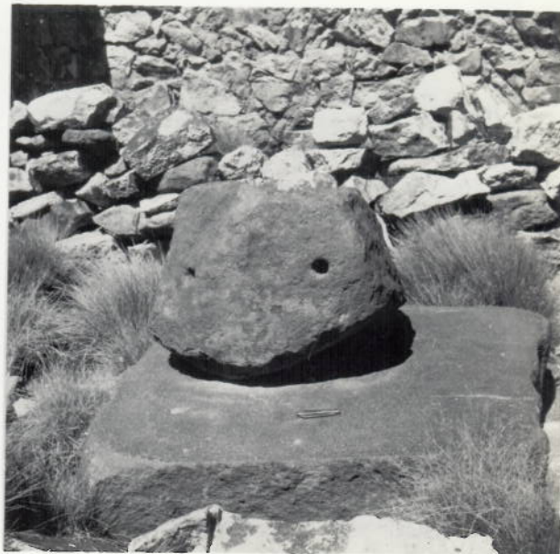
(18) "Boulder crusher" for crushing small pieces of ore. Note holes in boulder for wooden poles, used to promote rocking. Still in working order! Maccha Socaron.
