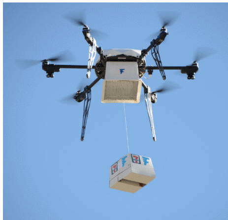
Figure 2.7: Flirtey Drone lowering its delivery on a winch(9)
