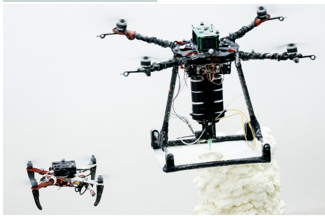
ScanDrone (left) monitors the progress of BuilDrone (right)
