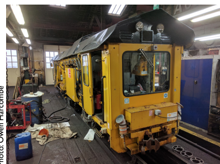
The tamping machine used to pack the ballast under the sleepers
