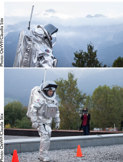
Back view of the equipped prototype showing base communications antenna (top). Mobility and visibility test (bottom).
