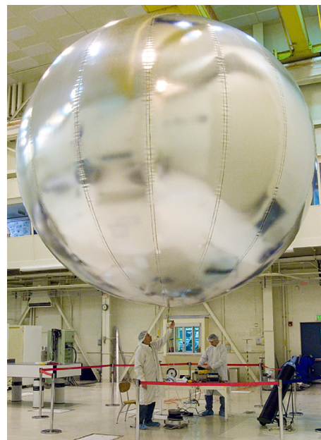
Figure 3: (Hall, Fairbrother, and Frederickson 2008) Prototype balloons showing the laminate fabric used - a clear layer of Teflon, bonded to metal foil and urethane undercoat for strength.
