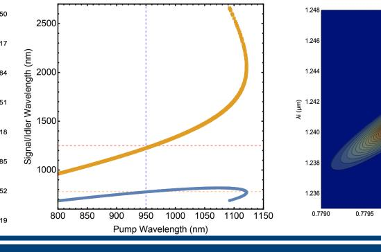
Spontaneous Four-Wave Mixing: 2 x Pump → Signal + Idler
