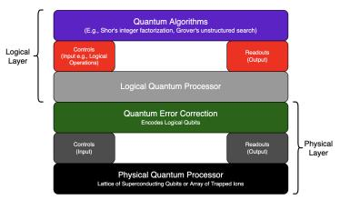
Systems overview of a fault-tolerant quantum computer with quantum error correction based on the creation of logical qubits from arrangements of physical qubits. Adapted from <sup>18</sup>
