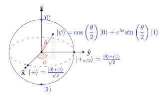
The Bloch Sphere, with the parameters  $\theta$  &  $\phi$  and showing states corresponding to each of the x, y, z axes for a single qubit.<sup>8</sup>
