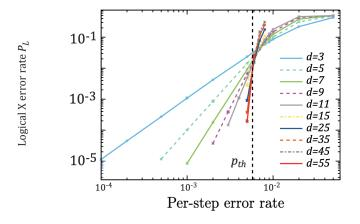
Experimental data has shown that the critical per-step error rate for the operating a Logical X is 0.57%. We see that once the per-step error rate is less than this the logical error rate decreases as we increase  $d.^{30}$
