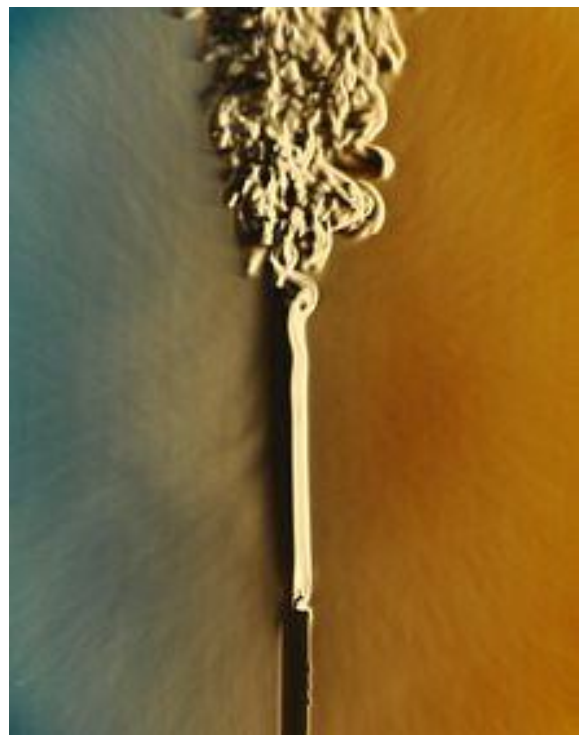
Figure 1, This exhibits the change from a laminar to turbulent flow in a candle flame. It arises when the external conditions generate the correct ratios of forces within the fluid. [5]
