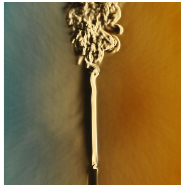
Figure 2. The plume from a candle is initially laminar, but transitions to turbulent flow in the upper third of the image. The Reynolds number can be used to predict where this transition occurs. (Settles, 2020)
