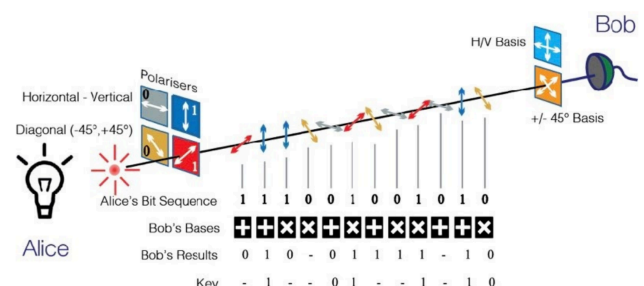
An example of how Alice and Bob could change bases to create a key using quantum key distribution. 14
