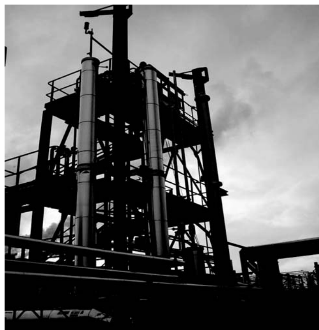
Fig. 3 RWE’s amine test rig at their Didcot combustion test facility. Commissioned in 2008, this plant has the capacity to treat 200 m 3 h -1 of flue gases and removes up to 1 tonne per day of CO 2 .
