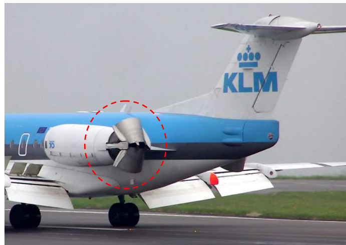
Figure 4.5. Reverse thrust engaged during a landing operation.
