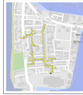
Figure 2.20 – London Heat Map, zoom on the Isle of dogs area (the existing network is drawn in yellow, the energy centre being represented by the green point [45]).
