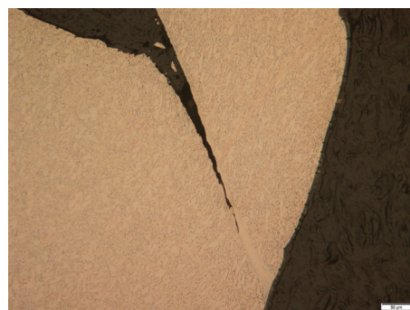
« Figure 14: Light microscopy image of a polished and etched fragment from a Ti-6Al-4V expanding cylinder, initial temperature 750K and a radial strain rate of 10^4 s^{-1} . Shown is an arrested fracture, propagating along an adiabatic shear band.
