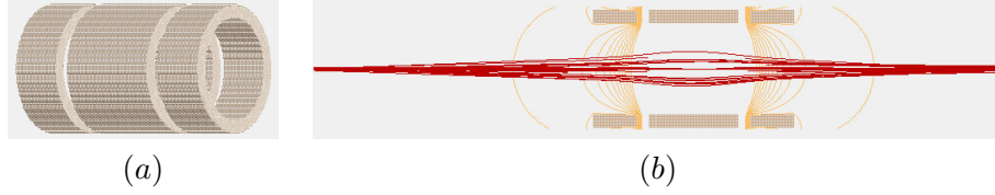
Figure 9.5: (a) an isometric and (b) cross-sectional view of the einzel lenses present in the SPECTRAP experiment. Potential contour lines (orange) and ion flight trajectories (red) can be seen in (b) for typical experimental parameters.
