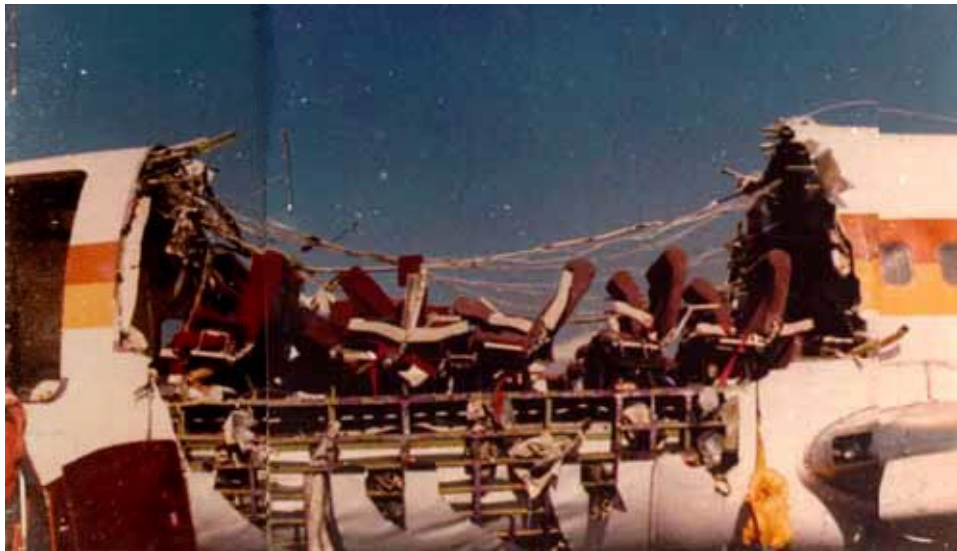
Figure 2.14 Photograph of Aloha Airlines 737, which suffered from a failure of the main fuselage lap joint.
