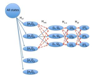
Figure 4: Effect of turning on the Hamiltonian  $\mathcal{H}_{hf}$ . Levels are split into states depending on F - note the small contributions to the states from other levels, shown in red. I have only drawn two other levels contributing for convenience, but all other levels will contribute in principle, even if they are in other terms and configurations. These states are still degenerate with respect to  $M_F$ .
